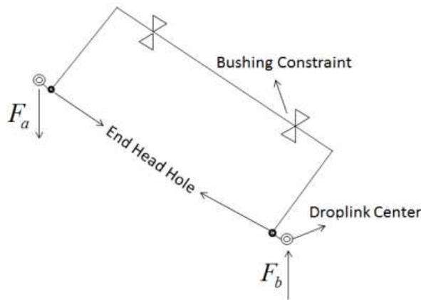
Fig. 2. The simplified forcediagramof the stabilizer bar
