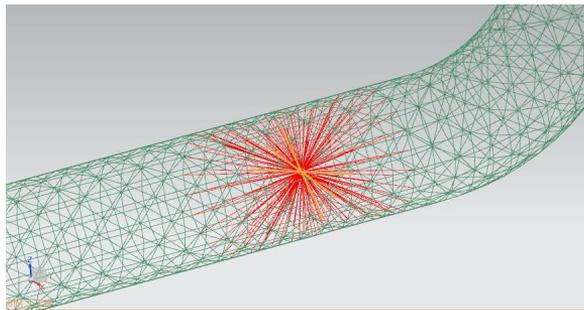
Fig. 4. RBE3 constraint of bushing contact area with bush stiffness
