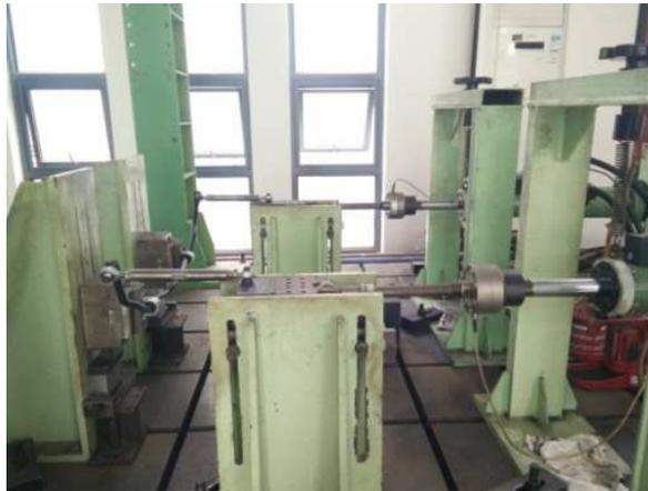
Fig. 10. Horizontal Fatigue MachineFig
