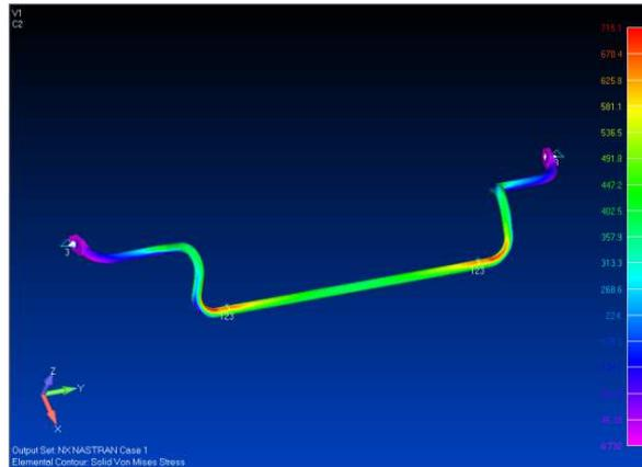
Fig. 6. Solid stress distribution of RBE2 constraint
