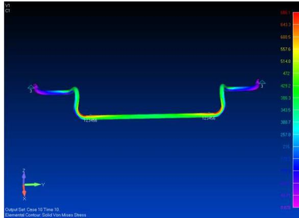
Fig. 7. Solid stress distribution of RBE3 constraint
